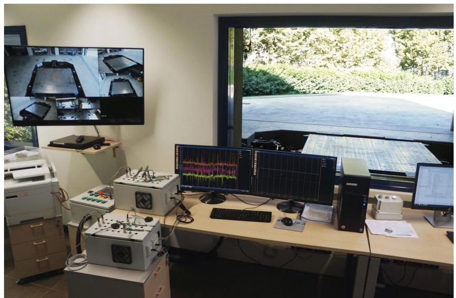
*Control room. From the window it is visible the vibrating platform on which the buildings are built in full scale for testing; on the monitors the iDaq interface is displayed.*
