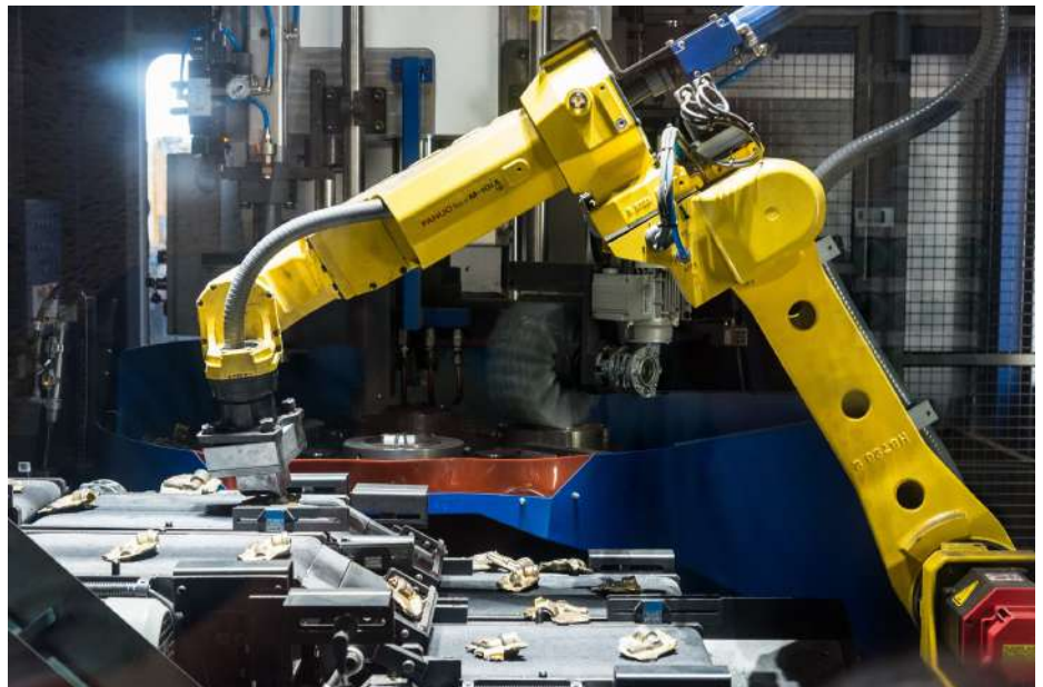
Robotic blanking of brass castings
